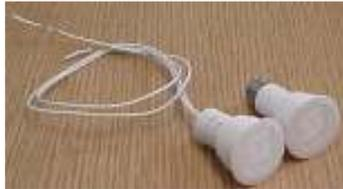
Other types of closed-loop door contacts may be used only in situations when the Sentrol 1078-C would not be practical. Every effort should be made to use a recessed door contact. Exceptions to this must be approved by the Office of Campus Computing prior to installation. See the door contacts appendix for more information.
