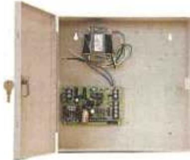
12/24 VDC, 4 amp switching power supply is agency listed for access control (UL 294 and CSA Certified). Features include field selectable voltage, power limited output, Form "C" relay fault reporting, visual fault indication and an additional output for Fire Alarm Interface (FAI). Systems integration applications include system power, door strikes, mag locks, card readers and fire alarm interface for emergency exit.
